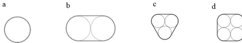
Fig.1. Design solutions for multifunctional pipelines for transporting oil, gas and water. Internal pipes can also be a combination of glass or basalt fiber.
